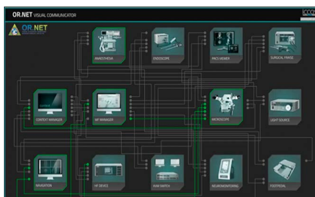
► Fig. 17 Network monitoring of medical assistance systems and data logging for sequential data storage of perioperative processes (figure taken from ICCAS Leipzig [80]).
