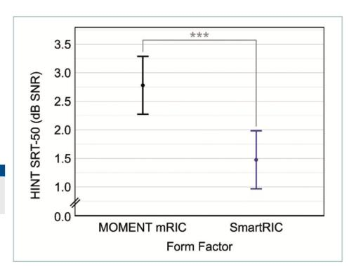
Results shows the SRT50 for each form factor. On average, the SRT50 measured with SmartRIC was about 1.25 dB smaller (or better) than that of the Moment mRIC.
