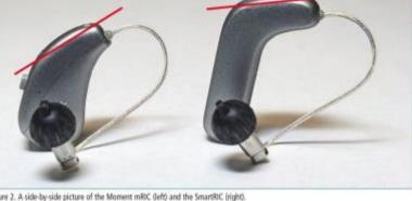
The current study showed that the design used in the SmartRIC hearing aid changed the microphone angle from an average of 37° (as in the mRIC) to an average of 12°, which significantly improved the SNR provided by the mRIC design used in the Moment mRIC hearing aid by 1.25 dB (from an average of 2.75 dB to 1.5 dB). It shows that it is possible to provide significative audiological improvement by working on the hearing aid mechanical design.
