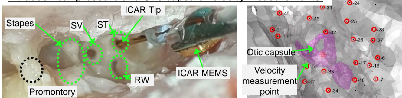
Fig. 2. Experimental access to intracochlear pressure (left), in scala vestibuli and tympany, and a proxy for the otic capsule motion, based on the 3D velocity of the medial skull surface (right), positioned within less than 2cm of the cochlear center.
