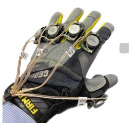
The Multichannel Vibrotactiles Gloves 1, 2 are designed according to the conceptual framework of Sharp (2023)
