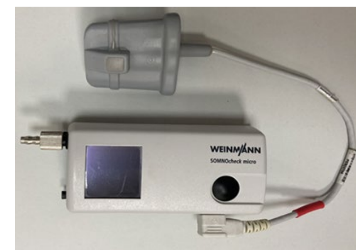
Fig. 1 – The HSAT device patients were examined with (Weinmann® somnocheck micro cardio device)
